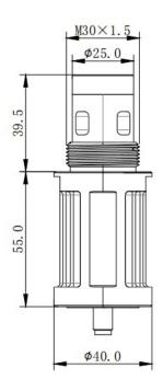
Unit: mm, Tolerance: ±0.5 mm
