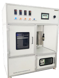
Fixed-Bed Catalyst Performance Evaluation System
